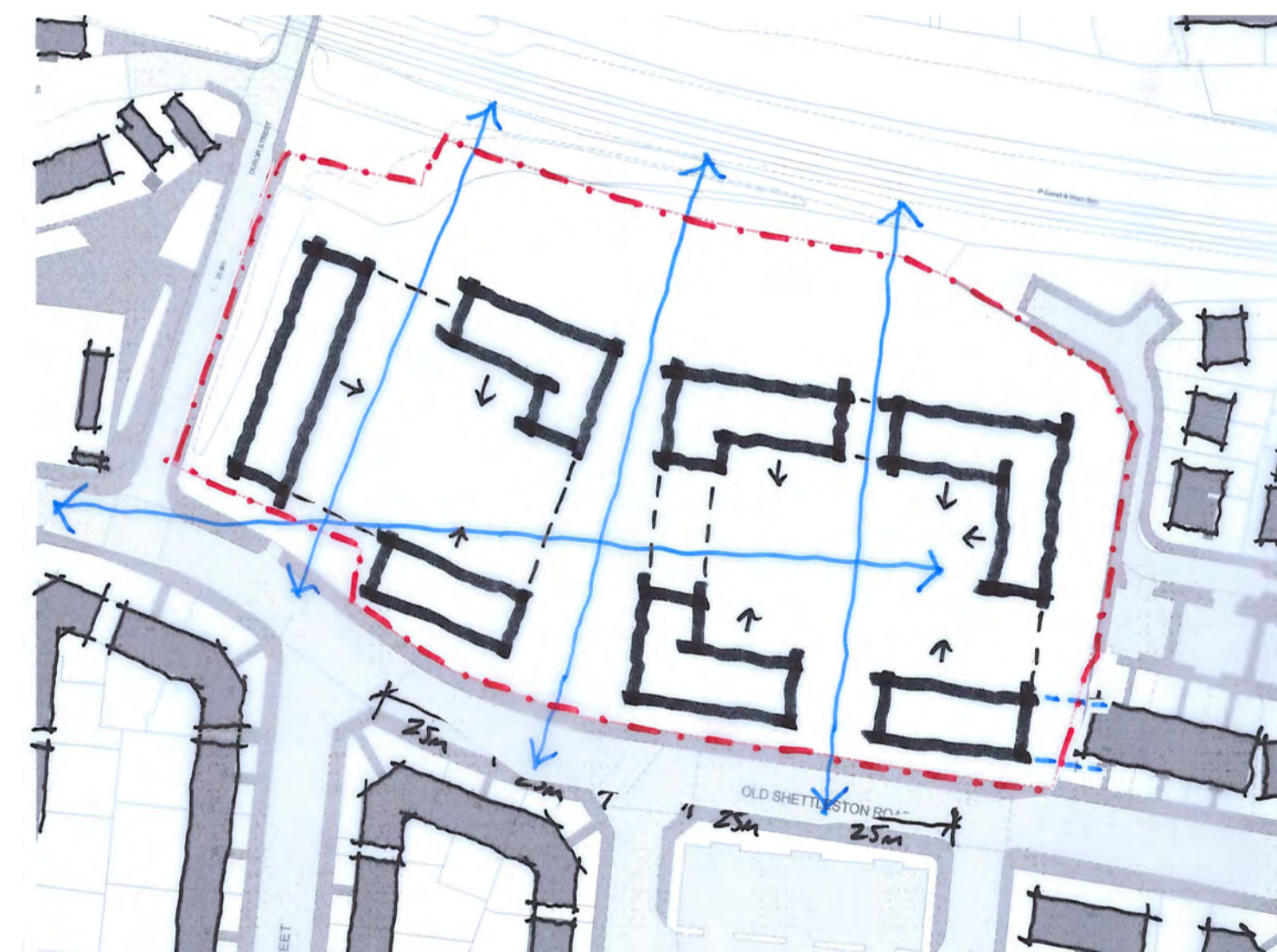
Creating courtyards and using key views through the site to articulate blocks and reduce massing.
